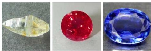
**Figure 1:** Three forms of  $\alpha\text{-Al}_2\text{O}_3$  with different doping, which affects optical properties: Corundum, Ruby and Sapphire.
