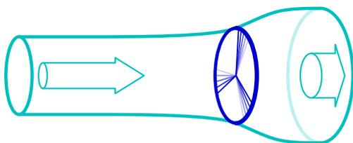
**Figure 8:** A wind turbine slows wind down and splays it out.
