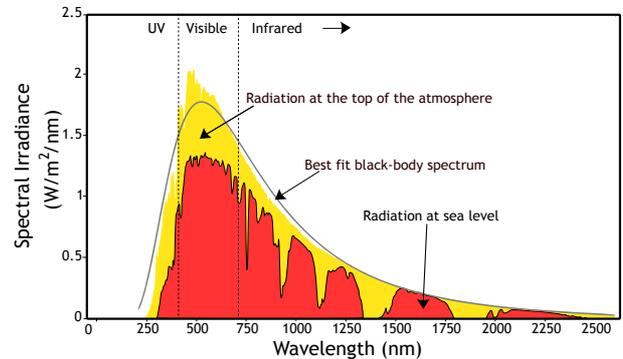
**Figure 3:** Spectrum of the Sun's light arriving at Earth. Yellow: Spectrum at the top of the atmosphere. Red: Spectrum at the surface of the Earth after atmospheric absorption. Black: best fit theoretical line.
