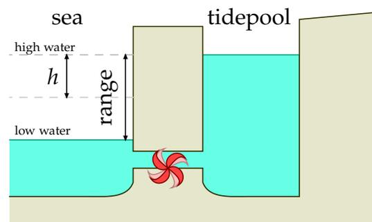
**Figure 16:** Cross-section of a tide pool. The pool was filled at high tide and now its low tide so we let the water out and generate electricity.
