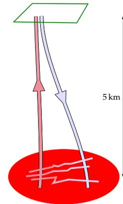
**Figure 20:** Harvesting geothermal energy by pumping cold water down one pipe then recovering it as steam via another pipe.
