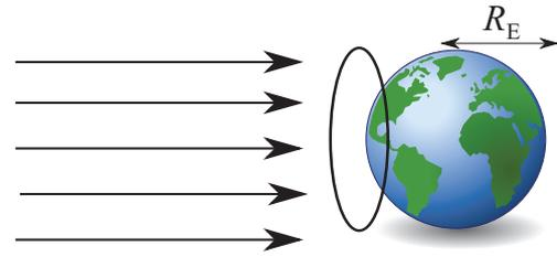
**Figure 21:** The solar energy hitting the earth (black arrows) delivers  $1300\text{W}/\text{m}^2$  of power, but the size of “net” the Earth has to catch this is only of area  $\pi R_E^2$ , while the actual surface of the Earth has area  $4\pi R_E^2$ .
