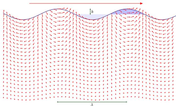
**Figure 15:** Diagram of a deep water wave. The top arrow indicates the speed of the wave, which is commiserate with the speed of the wind that generated it.
