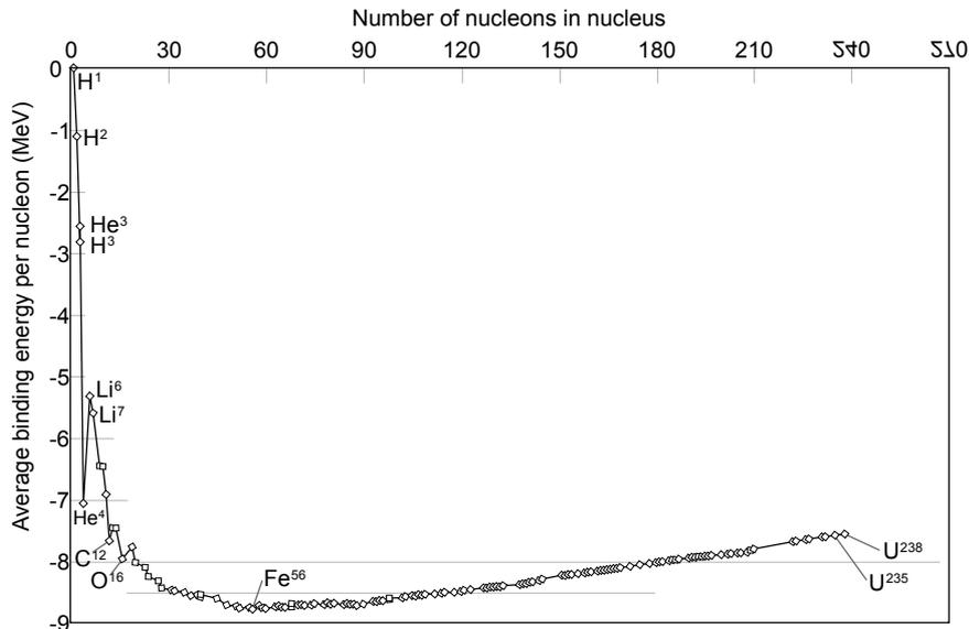
**Figure 24:** Nuclear binding energy per nucleon for a range of different atoms. Iron ( $Fe^{56}$ ) has the lowest energy per nucleon, so we can liberate energy either by splitting up atoms heavier than iron or joining together atoms that are lighter than iron.
