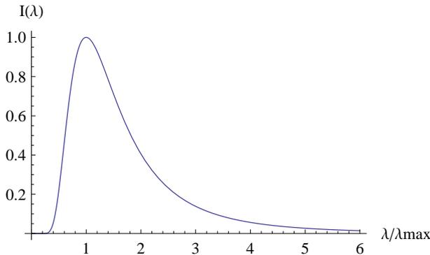
**Figure 2:** The power  $I(\lambda)$  radiated at each wavelength by a hot body. The spectrum is always the same shape, but hotter objects radiate with shorter wavelengths with  $\lambda_{max} = \frac{b}{T}$ , where  $b = 2.898 \dots 10^{-3}$  K m.
