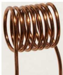
**Figure 71:** A wire coil forms an air-core inductor.
